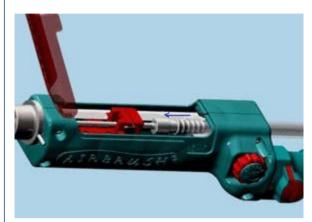
The Airbrush LiposculptureTM Intellimotion System consists of a small table-top controller and reciprocating cannula hand piece. The hand piece uses dual small air cylinders sequenced by the motion controller. Through a dual cannula arrangement, a smaller diameter cannula tube slides inside a larger diameter outer cannula.
